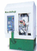
CNCホブ盤・小型ギア CNC hobbing machine for small gear sizes
