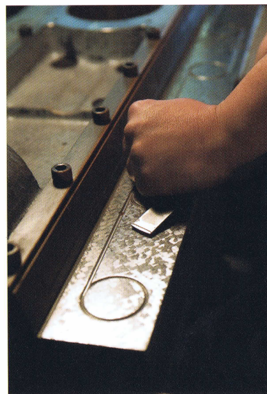
超精度のキサゲ加工 Ultra Accurate Hand Scraping of Machine Ways
